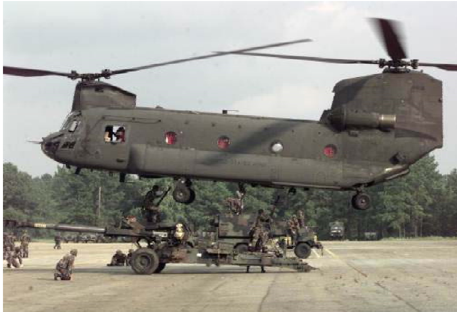
Figure 8A-1. CH 47D Lifting a 155 mm M198
