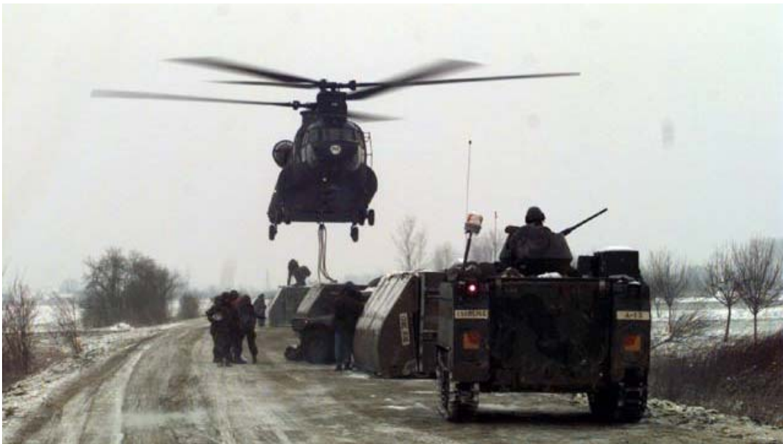
Figure 8-1. CH 47D Chinook Lifting Engineering Equipment
