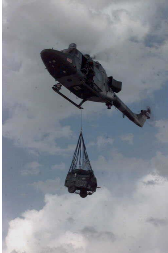
Figure 6-1. A Lynx Slung Load
